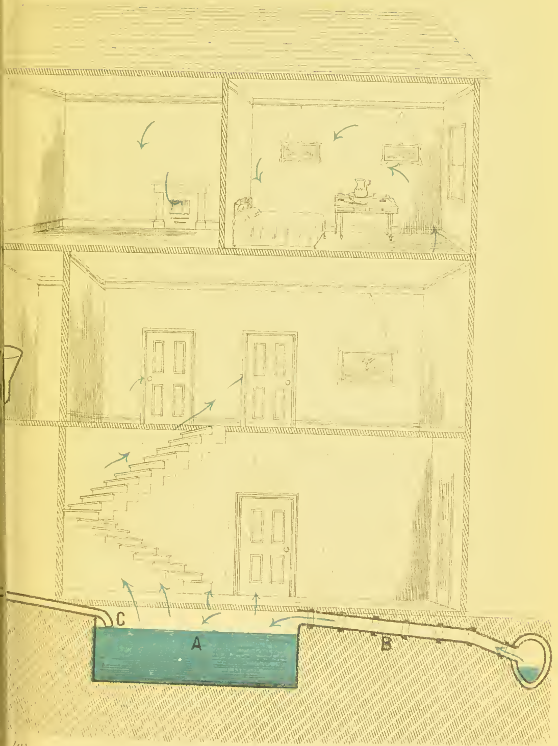
Rain water tank under cellar floor, overflow into drain.
